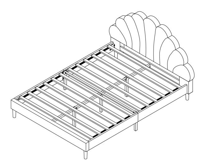
\* When moving the bed position, the center support legs must be adjusted or straightened to avoid any broken problems.
