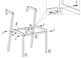
Step 2-Use screws(Part H) to connect the chair metal frame with the backrest(Part A)
