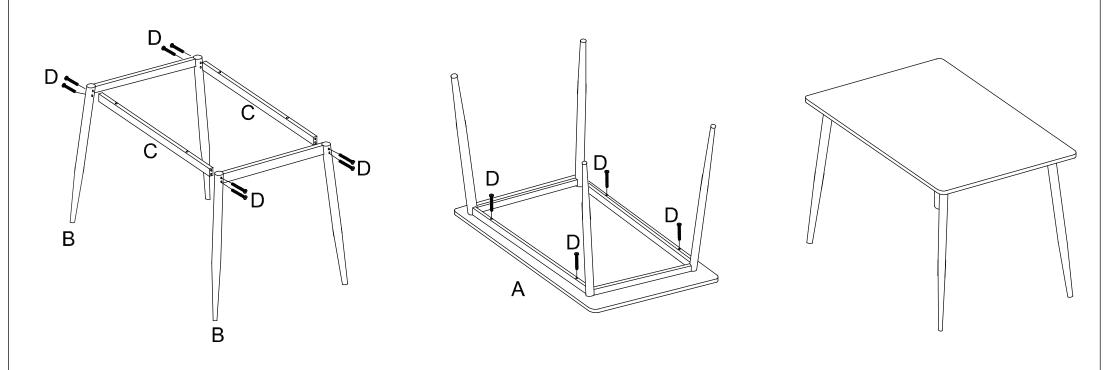
Step 1-Use screws(Part D)to connect cross-bars (Part C) with table feet(Part B) as table metal frame
