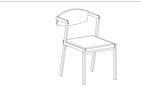
Step 1-Use screws(Part H/J)to connect chair feet(Part C/D) with cross-bars (Part F) Insert G into the holes of Part F and Part E,
