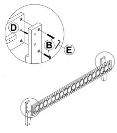
Attach the footboard post (P5) to the footboard panel (P4) using hardware:
