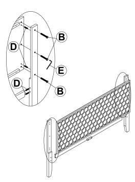
Attach the headboard post (P3) to the headboard panel (P1) and headboard bottom rail(P2)
