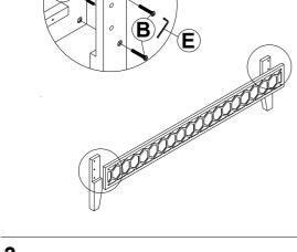
Attach the side rail (P6) to the headboard post (P3) and footboard post (P5) using hardware:
