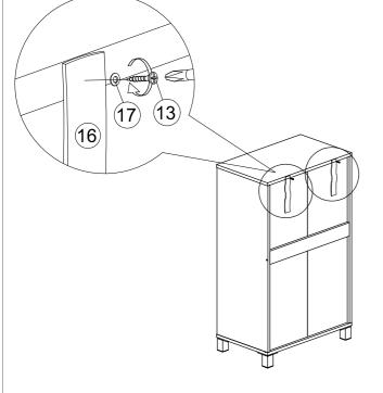
4. Add safety strap (16), washer (17) using 3.5x15mm screw (13) to back of cabinet.
