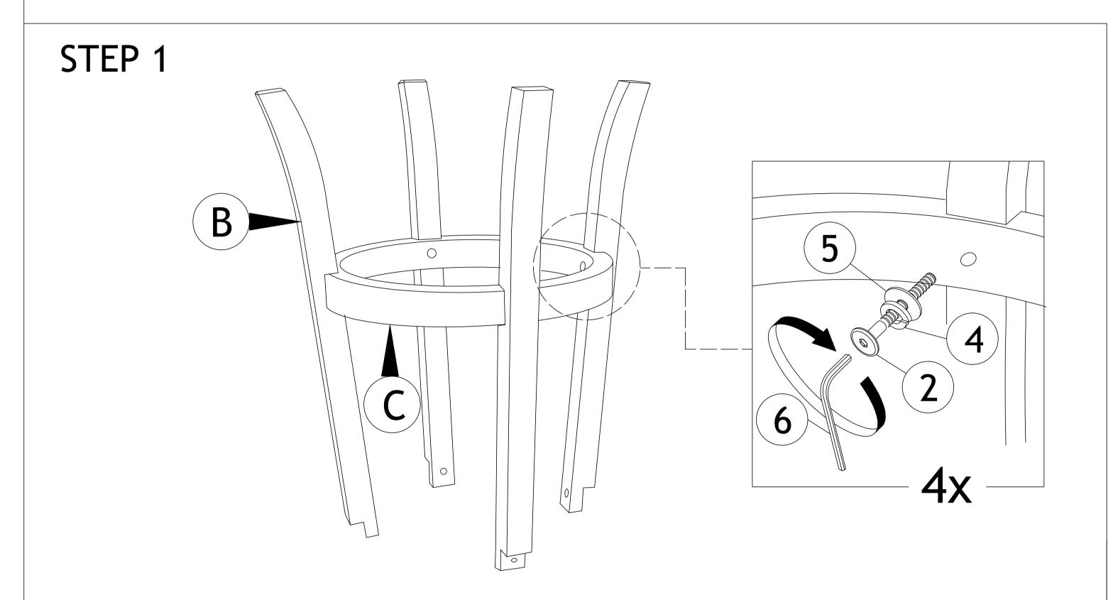
Attach part(B) with part(C). Insert each individual set of hardware as per picture shown. Do not tighten any hardware completely.
