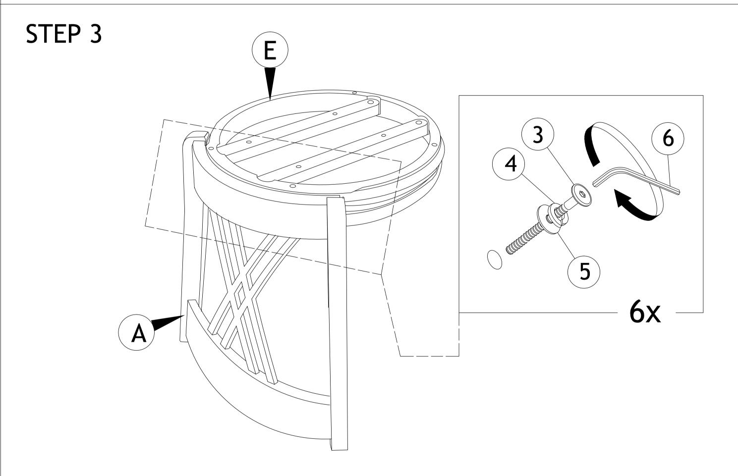
Insert 6 sets hardware first, then tighten part(A) with part(E) completely after alignment is done.
