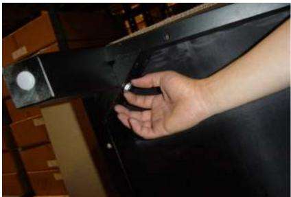
Step 3 Use the nut to tighten the inside.
