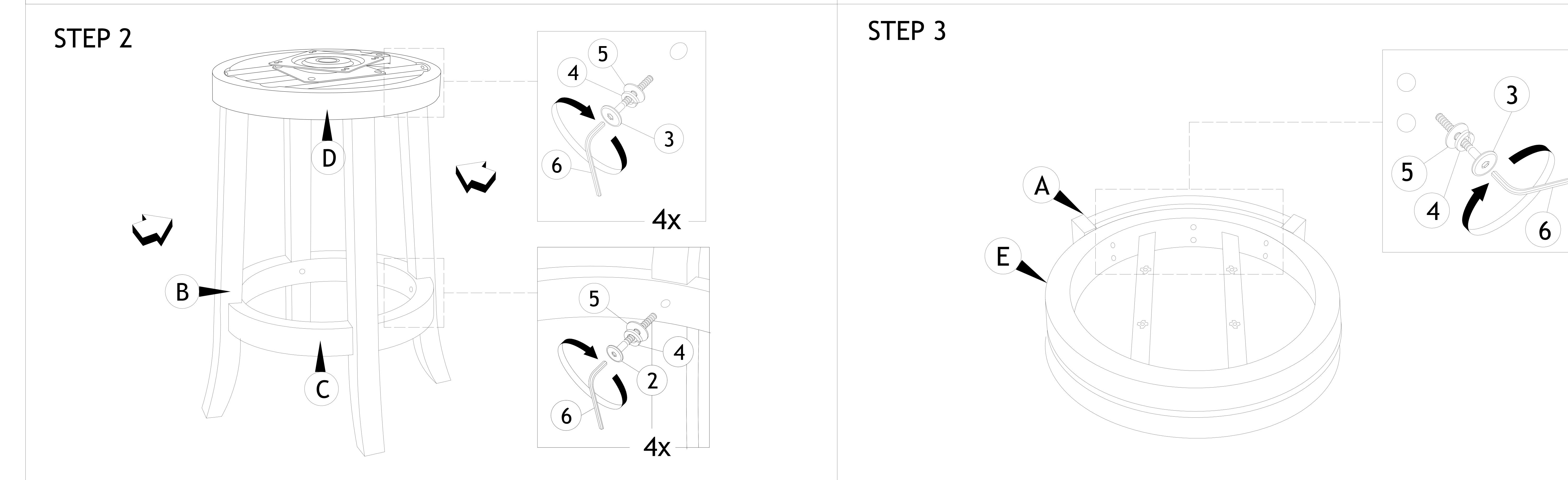
Attach part(B) with part(D). Tighten part(B) with part(D) first, then tighten part(B) with part(C) completely. Insert 6 sets hardware first, then tighten part(A) with part(E) completely after alignment is done.
