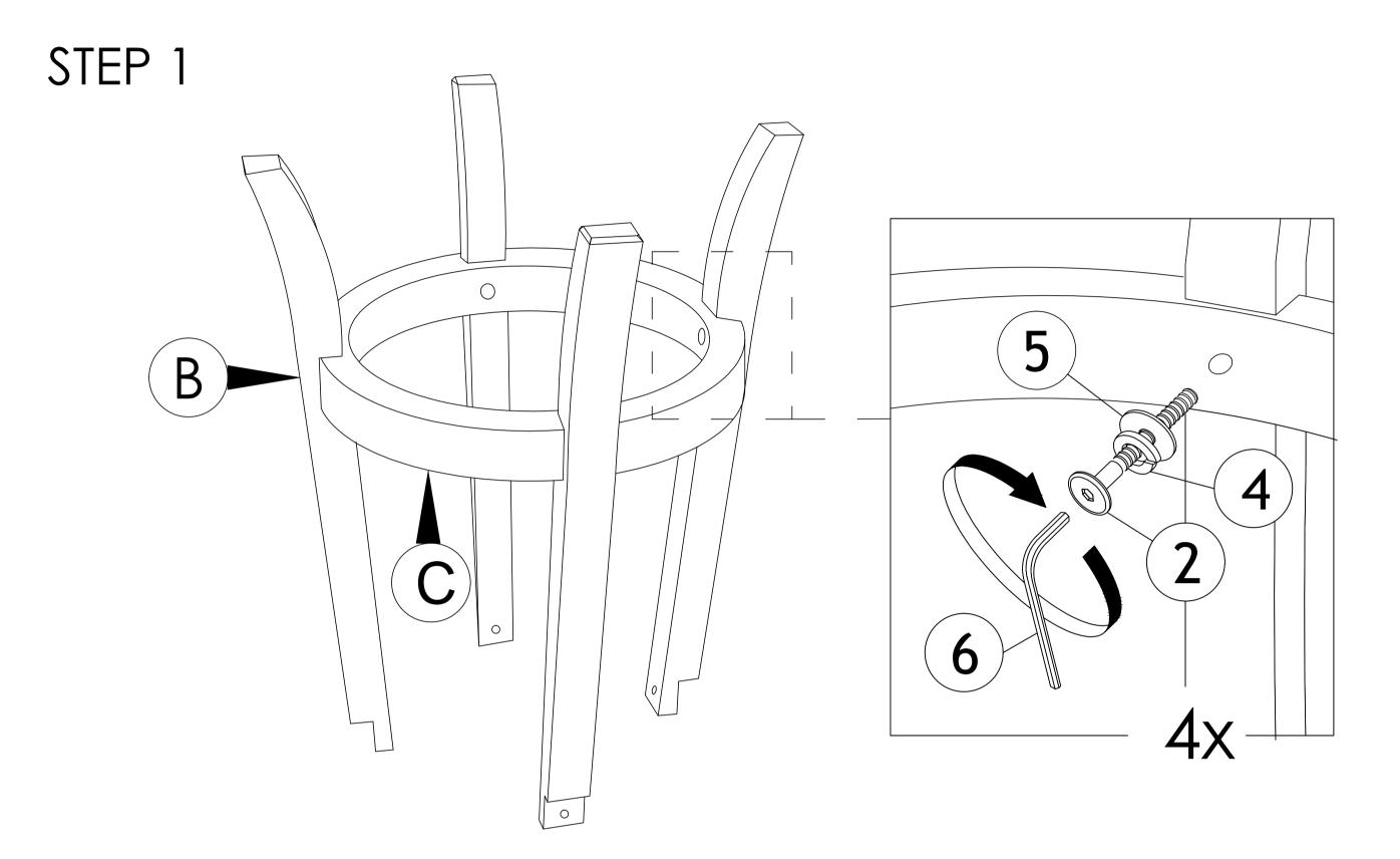
Attach each leg (B) to footrest (C). Insert each individual set of hardware as per picture shown. Do not tight up any hardware completely.
