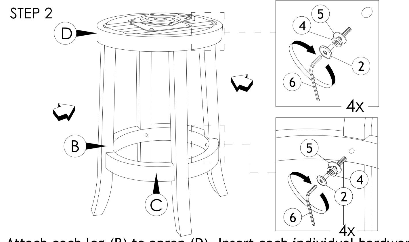
Attach each leg (B) to apron (D). Insert each individual hardware as per picture shown. Tight up 4 legs with apron first, then tight up footrest with 4 legs completely.
