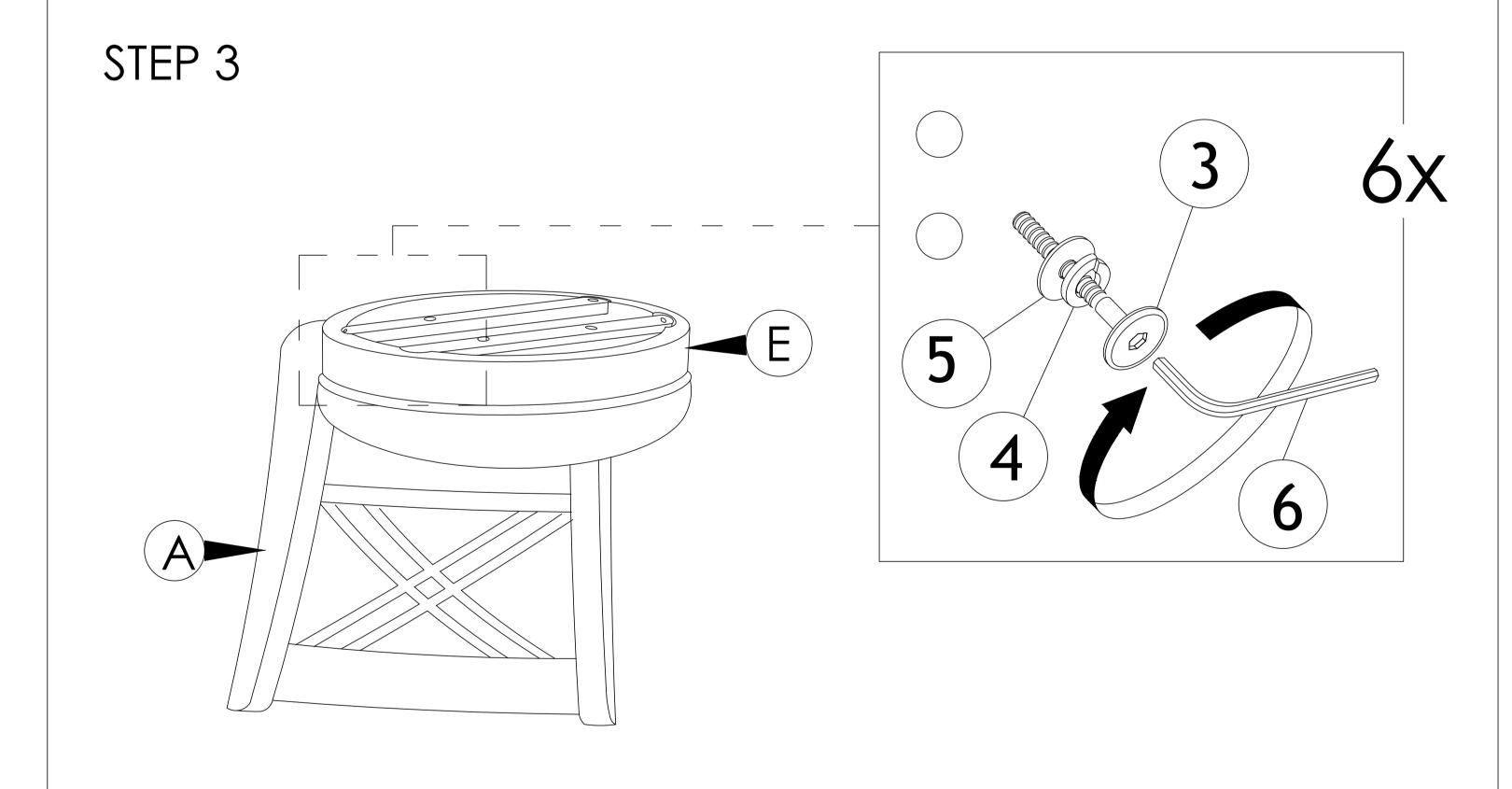
Insert 6 sets hardware first, then tight up part (A) with part (E) together after alignment is done.
