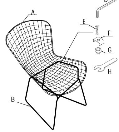
Keep the holes of the seat pannel and Leg in line, use the M6screw to reinforce only.
