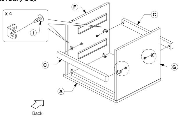
9 Slide the Back Panel (D) into the groove on the back of the Side Panel (F & G).
