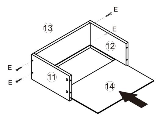
Connect board 13 to 11&12 with screw E Slide board 14 into the grooves 11&12&13
