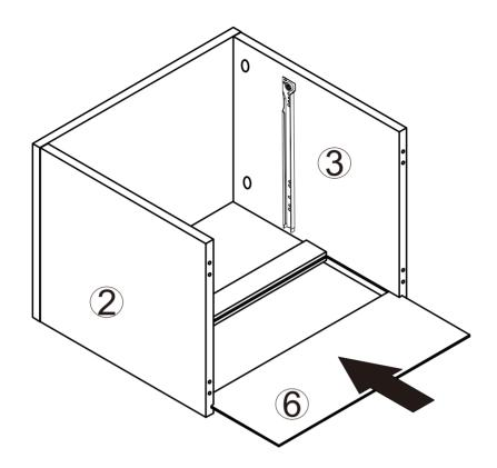
Slide board 6 into the grooves of 2&3&5
