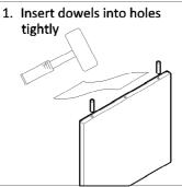
2. Attach the insert holes along with dowels
