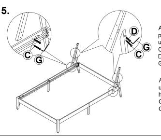
Attach the headboard lower post (P2) to the headboard upper post (P1) using hardware:
