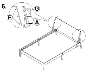
Attach the headboard panel (P3) to the headboard upper post (P1) using hardware:
