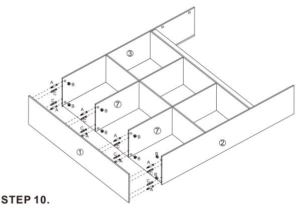
Insert quickfit screws (A) into part 5, as shown. Insert cam locks (B) and wooden dowels (C) into part 10, as shown.
