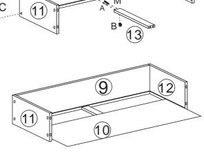
STEP 3. Insert quickfit screws (A) to parts 14. And fix handles (H) to parts 14 using screws (E), as shown. Insert cam locks (B) and wooden dowels (M) to parts 11, 12 and 13, as shown. Attach parts 14 to assembled drawers.
