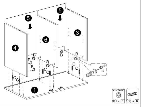
Insert wooden dowels (C) into parts 4, 6 and 3.
