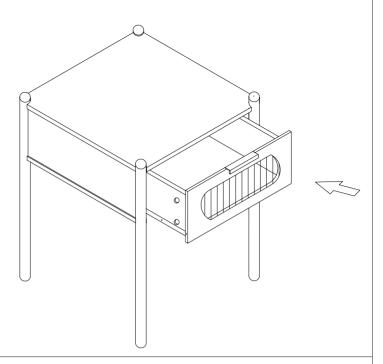
10 Put the plastic corner support (H) on the backboard 5 using screws (I). The unit should now be assembled and ready to use.
