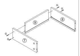
2 Slot piece 10 into the ridges. First insert the cam locks (B) into the pre-drilled holes on parts 7 & 8. Line up these screws with the pre-drilled holes on the front piece 6. Once attached, tighten the cam locks (B) using a cross-head screwdriver and ensure the piece is secure.
