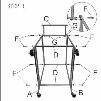
Place the metal legs(A,B) to a soft surface,and fasten the handle(C) and metal side parts(D), by using nuts (F,G) with wrench.
