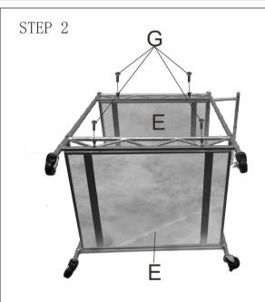
Attach the top and bottom shelves(E) to the assembled parts.
