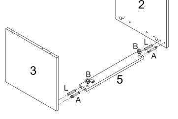
Then attach piece 1 using wooden dowels (L), cam dowels (A) and cam locks (B), tighten the cross dowels.
