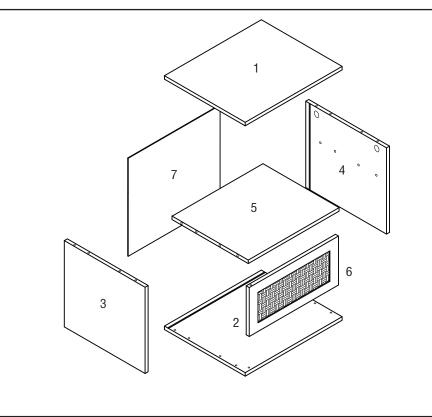
Attach piece 3 & 4 to piece 5 using wooden dowels (C), cam dowels (A) and cam locks (B).
