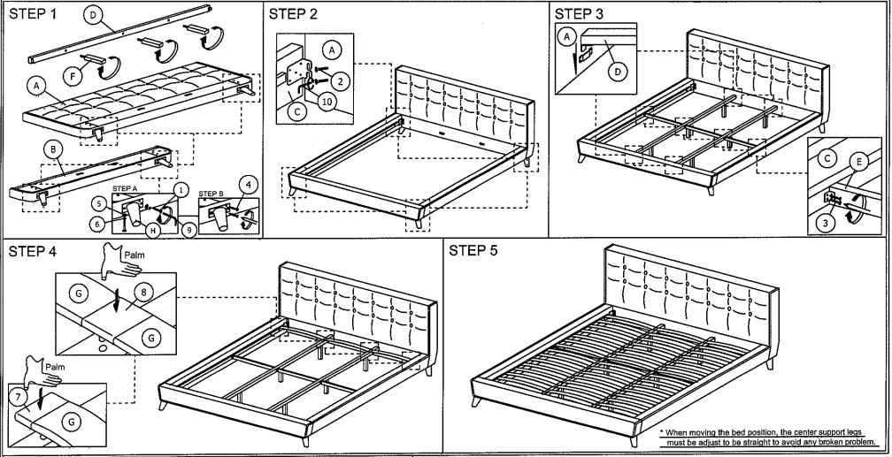
CAUTIONS : 1. Do not FULLY - TIGHTEN the nut or nut bolt until all nut or bolt is ready assembed. 2. Do not OVER - TIGHTEN the nut or bolt to avoid causing damages to the thread. 3. Keep all hardware parts out of reach of children.
