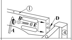
Step 4 Use hardware D to locate part 5 on the assembled seating frame as shown, and fully tighten it with hardware C.
