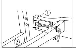
Step 3 Attach part 4 with the assembled part 1, and lock it using hardware A,B,D,and E.
