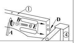
Step 4 Use hardware  $\underline{D}$  to locate part  $\underline{5}$  on the assembled seating frame as shown, and fully tighten it with hardware C.
