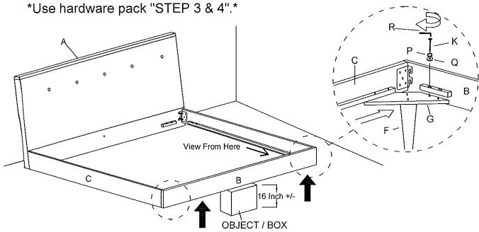
Level up the Headboard Panel (A) by putting on object/box to fix the Bed Leg (F) with the Bed Leg Support (G). Insert JCBC M6 X 50mm (K) Flat Washer M6 (Q) Spring Washer M6 (P) to Headboard panel (A) connection Bed Leg Panel by Allen Key M4 (R).
