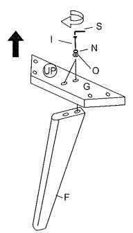
Insert JCBB M8 X 25mm (J) Flat Washer M8 (O) Spring Washer M8 (N) to Side Rail (C) connection Hb/Fb panel (A/B) by Allen Key M5 (S).
