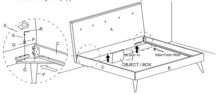
[5] Insert JCBC M6 X 15mm (L) to L/Bracket (U) to connection Center Support (D) by Allen Key M4 (R).
