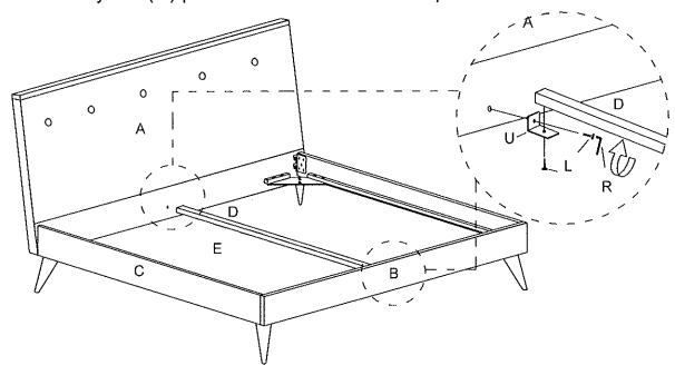
Insert JCBC M6 X 70mm (M) into the Center Support (D) by Allen Key M4 (R) into the Support Leg (E), and turn the Adjuster M6 (T) into the bottom of the Support Leg (E).
