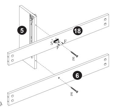
Fix maget on board (18) with screw (F).Lock shelf board(6) to divider panel(5) with screw(E).
