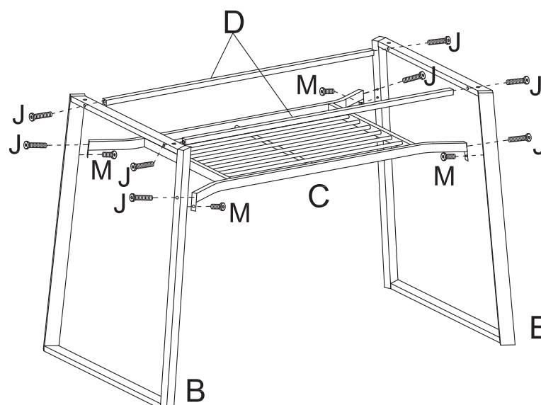
**2** step 2-Use screws(Part L)to connect table metal frame to the table top (Part A)
