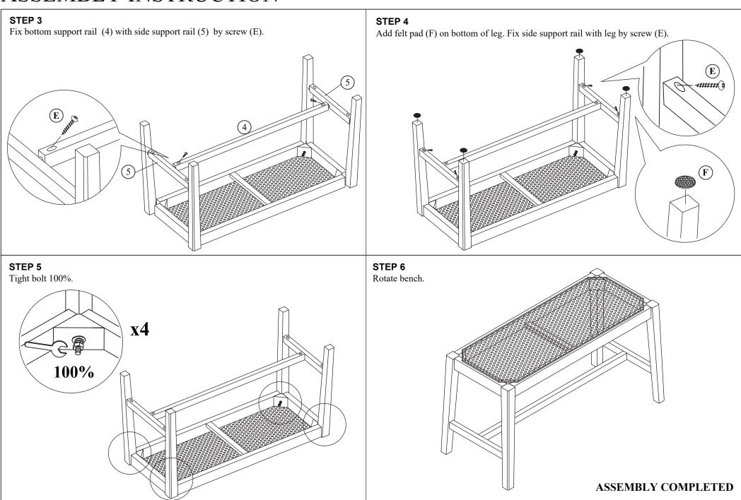
NOTE: AFTER A FEW DAYS OF ASSEMBLY. IT WILL HAVE ACCLIMATIZED TO THE ENVIRONMENT. PLEASE TIGHTEN ALL HARDWARE.CHECK TIGHTNESS OF
