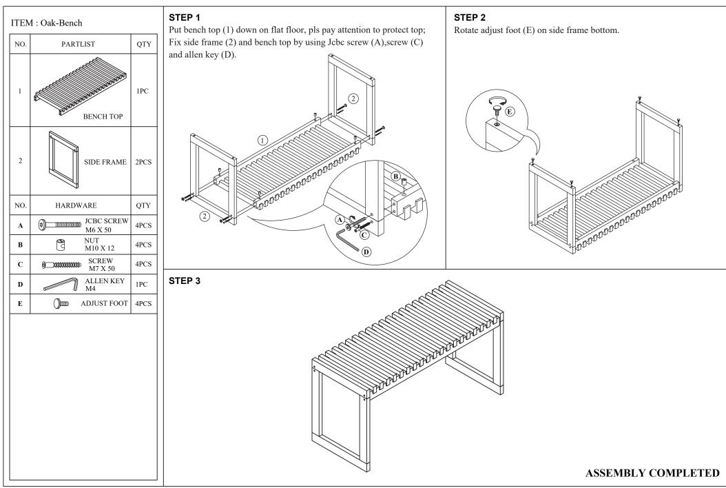
NOTE: AFTER A FEW DAYS OF ASSEMBLY. IT WILL HAVE ACCLIMATIZED TO THE ENVIRONMENT. PLEASE TIGHTEN ALL HARDWARE.CHECK TIGHTNESS OF ALL SCREWS EVERY 6 - 8 WEEKS.
