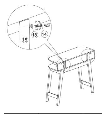
4. Add safety strap (15), washer (18) using 3.5x16mm screw (14) to back of cabinet.
