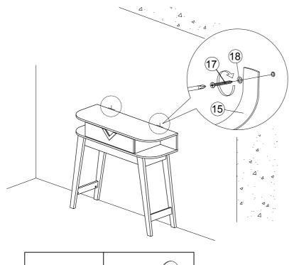
5. Finally, attach safety strap (15) and washer (18) using 4x30mm screw (17) to the wall.
