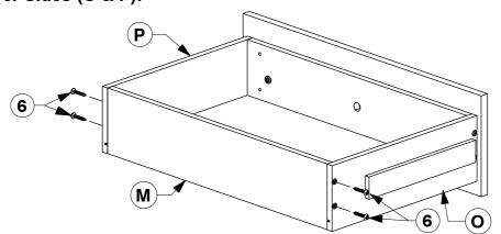
Turn the Drawer over to fit angled 25mm Wood screws (6) to the Drawer Rail (N).
