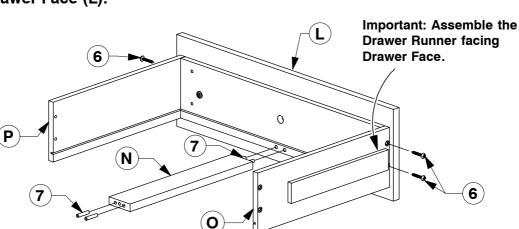
4 Slide the Drawer Bottom (K) into the groove on the Drawer Sides (O & P).
