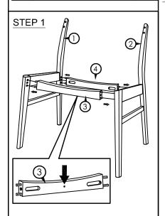
Front Stretcher (3) has a small hole for identification.
