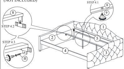
Please do not tighten the hardware until the entire assembly is completed.
