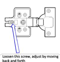
● There is a gap on the top of the door when doors are closed (Glass slide hinge does not require this step)
