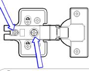
② Adjusting screw (If you twist clockwise once, the door moves about 2mm inward)
