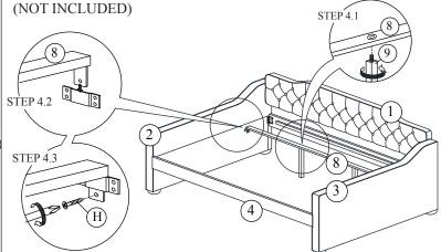
Please do not tighten the hardware until the entire assembly is completed.
