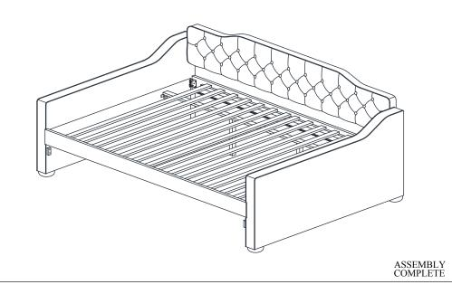
Please do not tighten the hardware until the entire assembly is completed.
