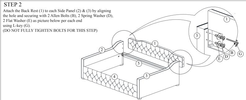
Please do not tighten the hardware until the entire assembly is completed.
