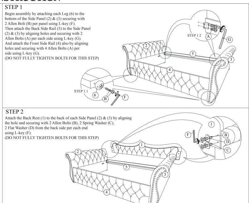
Please do not tighten the hardware until the entire assembly is completed.
