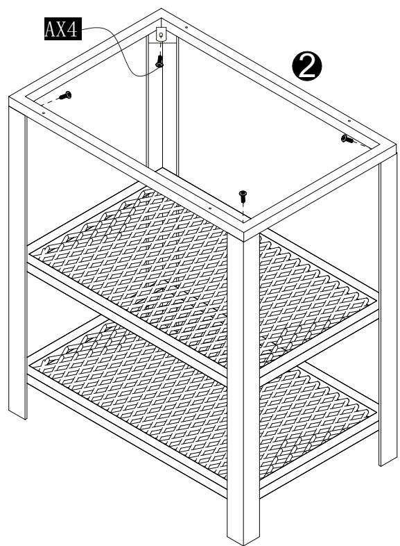
· Fix the 4 part to the 3 part with the hardware A.
