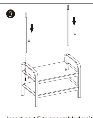
Insert part E to assembled unit with screw a.
