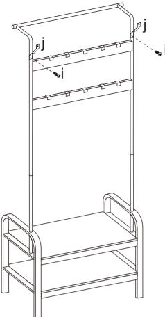
·Connect Part J to the assembled unit with screws i.
