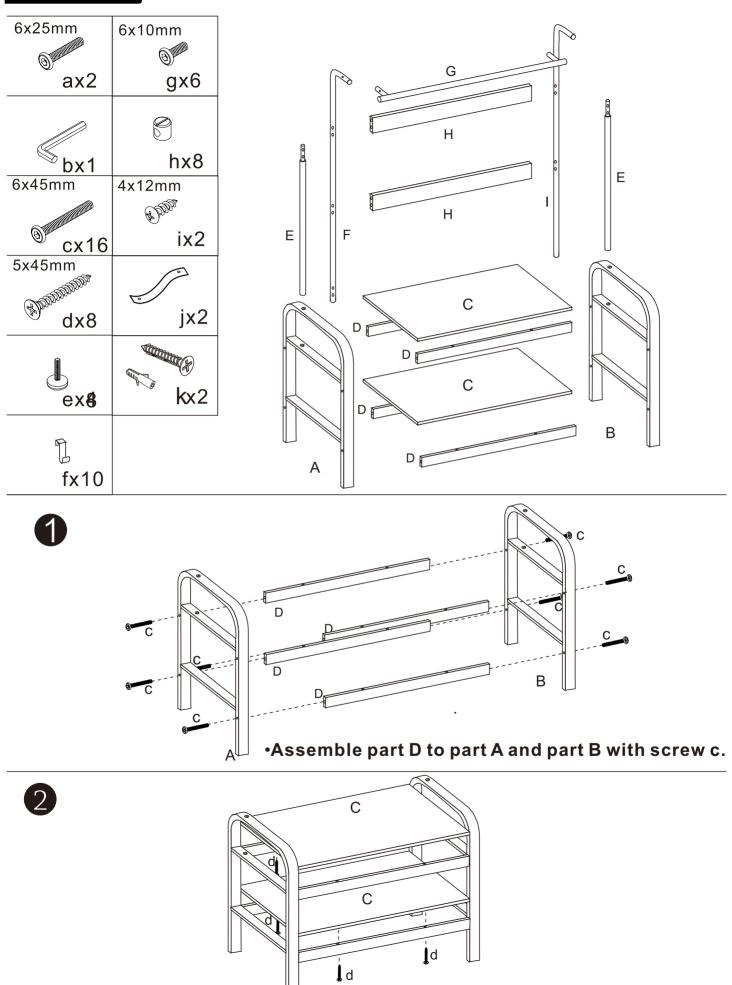
Insert part C to assembled unit with screw d as shown
