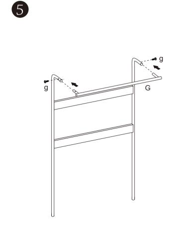
Insert G part to the assembled unit with screw g.
