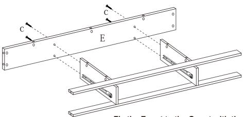
Fix the E part to the G part with the hardware c.
