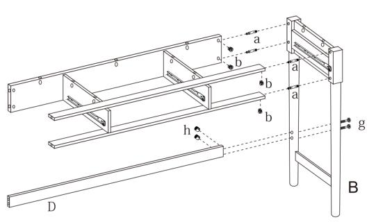
Fix the B part to the D/E/F part with the hardware a/b/g/h.
