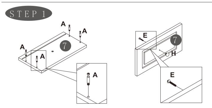
Insert hardware A to part 7 as shown Attach hardware H to part 7 using hardware E
