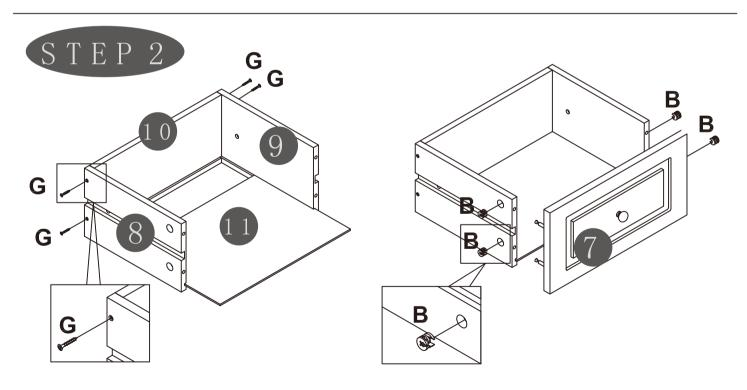
Assemble part 10 to part 8 and part 9 with hardware G Insert part 11 to assembled unit as shown Assemble part 7 to assembled unit by using hardware B
