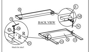
Step 3: Attach the JCBB Bolt (J) to the headboard bracket and footboard bracket .
