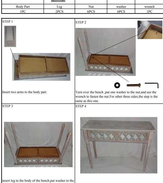
nut then add it to the hole of the leg, at last use the wrench to fasten the screw. For other three legs, the step is the same as this one
