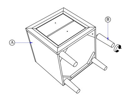
STEP 2: Reinstall handle by loosen the handle screw then tighten up as shown.
