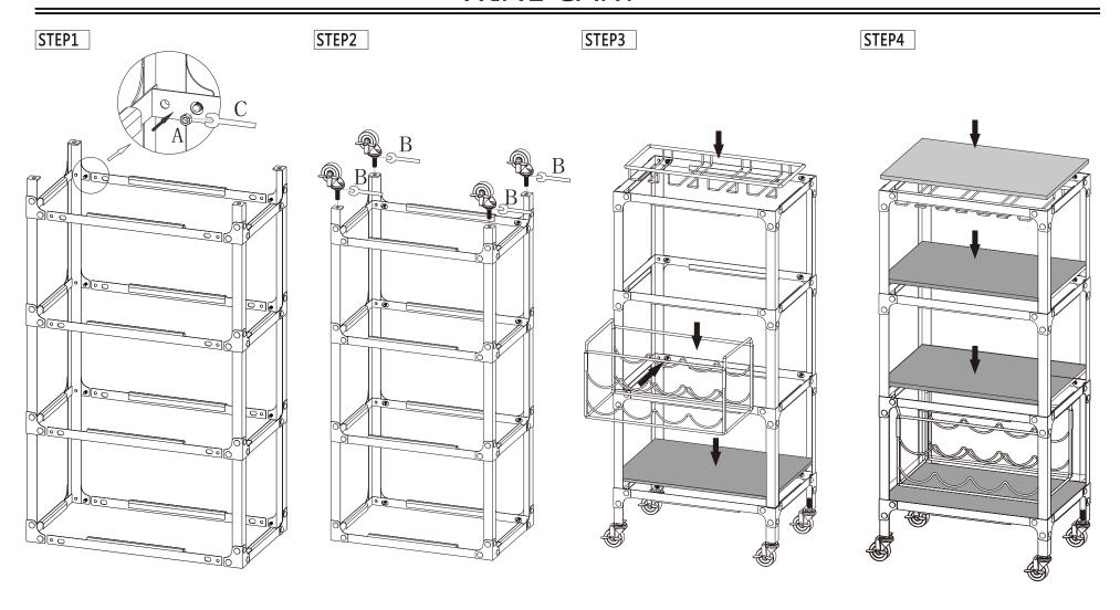
Note: Pls do not tighten all bolts until the products is assembled completely.
