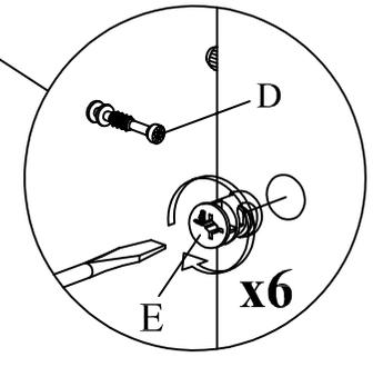
\*Assemble right side panel (4), secure with Minifix as shown.
