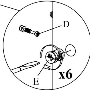
\*Assemble left side panel (2), secure with Minifix as shown.
