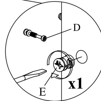
**\*Assemble middle support leg (12), side legs (13) secure with Minifix as shown.**
