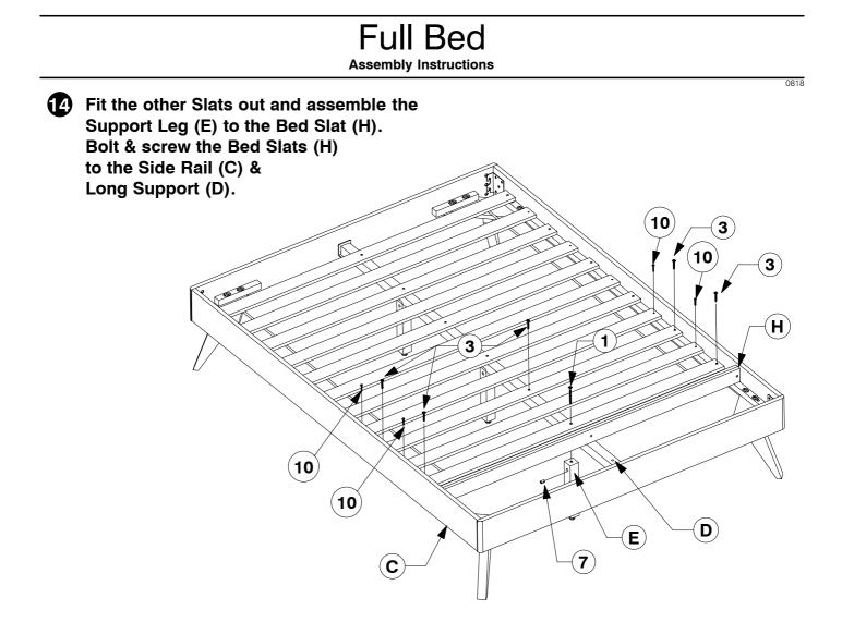
**Bolt & screw the remaining Bed Slats (H)** to the Side Rail (C).
