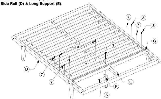
Bolt & screw the remaining Bed Slats (G) to the Side Rail (D).
