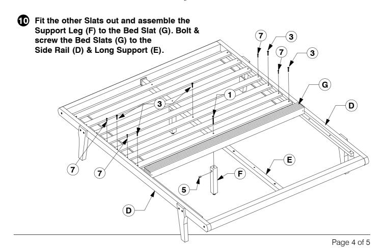
Fit the other Slats out and assemble the Support Leg (F) to the Bed Slat (G). Bolt & screw the Bed Slats (G) to the Side Bail (D) & Long Support (F)
