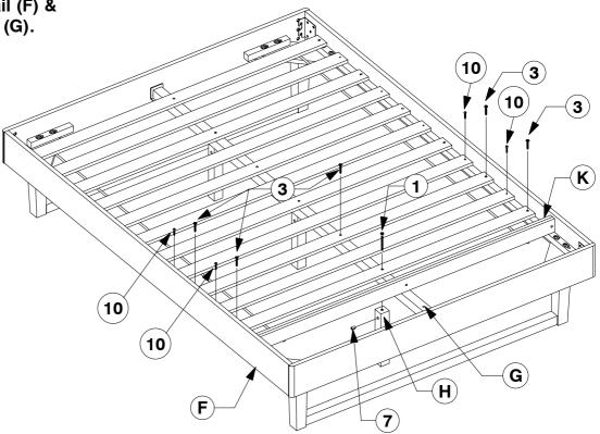
Bolt & screw the remaining Bed Slats (K) to the Side Rail (F).
