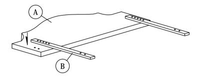
Align pre-drilled support stand holes over the pre-drilled headboard holes according to your desired headboard height
